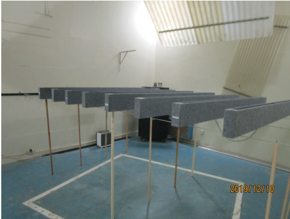
Figure 1 – Specimen mounted in test chamber
