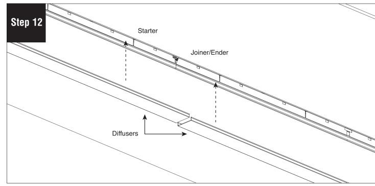
Reinstall diffusers to starter and joiner/enders and turn power on to luminaire. **NOTE**: If part of a longer run, diffuser will be reinstalled back into original luminaire section as lengths vary.
