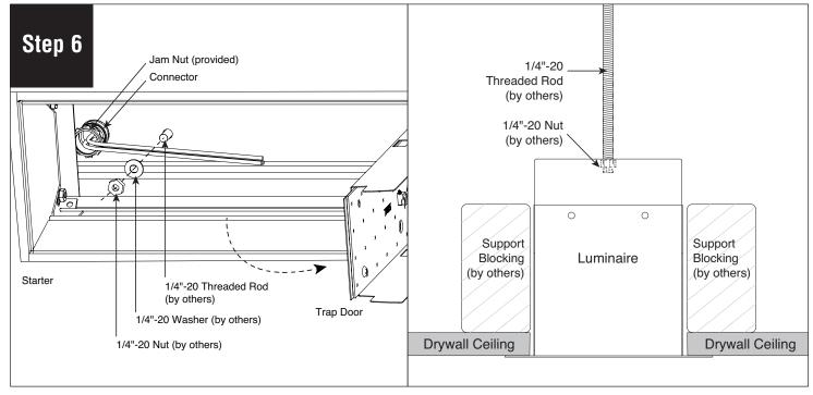
**ALTERNATE MOUNTING OPTION** Support Blocking (by others) Screw (by others) Support Support Blocking Blocking (by others) (by others) Luminaire (by others) Trap Door **Drywall Ceiling Drywall Ceiling**
