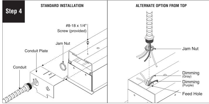
Remove jam nut from conduit then insert wires and connector through feed hole.
