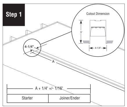
Add 1/4" to body/row length (A), +/- 1/16" to simplify installation. Luminaire needs to be installed next to support blocking.
