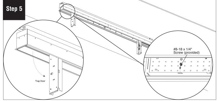
Remove #8-18 x 1/4" screw (provided) to open trap door and then insert luminaire into ceiling. Align luminaire within rough opening in drywall and 1/4"-20 threaded rod (by others).
