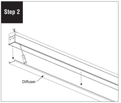
Remove diffuser and set aside to prevent from getting dirty or damaged. **NOTE:** If part of a longer run, diffuser will be reinstalled back into original luminaire section as lengths vary
