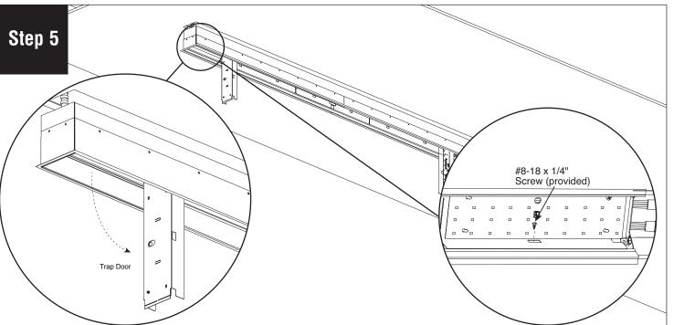
Remove #8-18 x 1/4" screw (provided) to open trap door and then insert luminaire into ceiling. Align luminaire within rough opening in drywall and 1/4"-20 threaded rod (by others).
