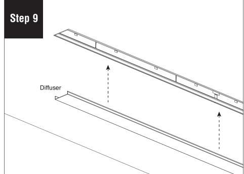
Reinstall diffuser and turn power on. **NOTE:** If part of a longer run, diffuser will be reinstalled back into original luminaire section as lengths vary.
