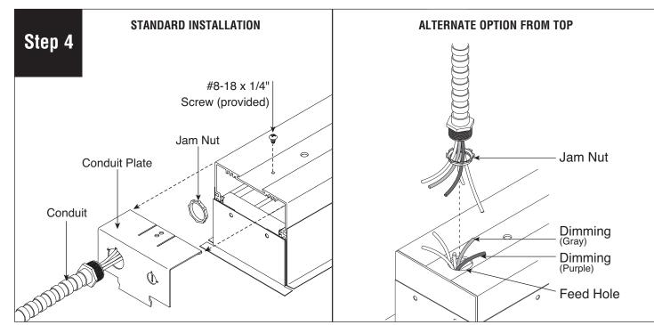
Remove jam nut from conduit then insert wires and connector through feed hole. NOTE: Purple and gray wires are for Low Voltage Control.
