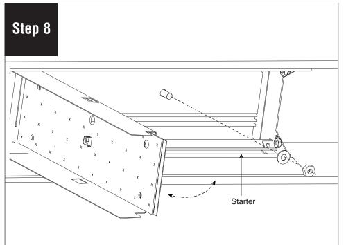
On opposite end of luminaire, fold trap door down. Install 1/4"-20 nut (by others) and 1/4" washer (by others) onto 1/4"-20 threaded rod (by others) or use ALTERNATE MOUNTING OPTION in step 6. Replace trap door and fasten with #8-18 x 1/4" screws (provided).
