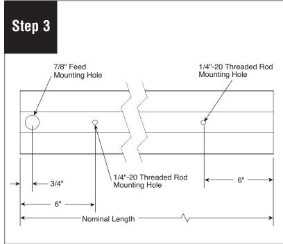
Refer to threads and feed hole locations above before connecting luminaire wires.
