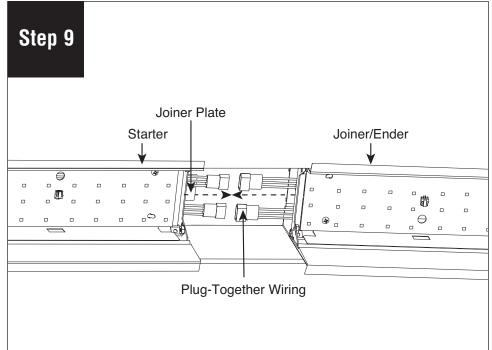
Connect plug-together wiring. Slide joiner luminaire against starter luminaire Be careful not to damage any wiring.
