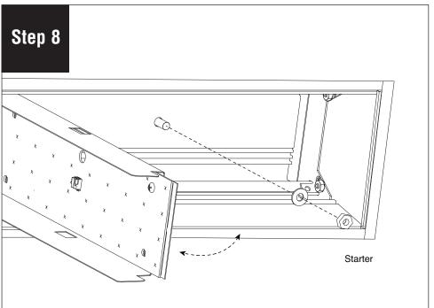
On opposite end of luminaire, fold trap door down. Install 1/4"-20 nut and 1/4" washer onto 1/4"-20 threaded rod (by others) or use ALTERNATE MOUNTING OPTION in step 6. Replace trap door and fasten with #8-18 x 1/4" screws (provided).
