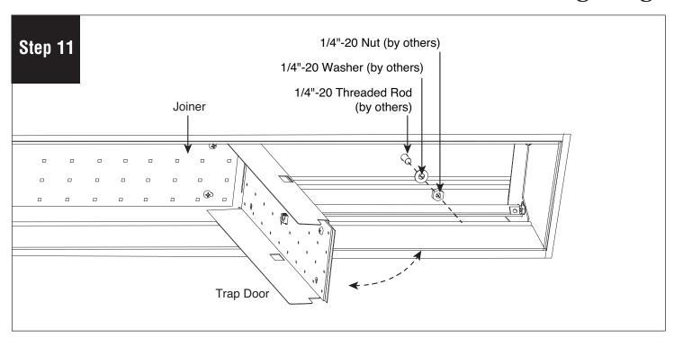
On opposite end of luminaire, fold trap door down. Install 1/4" washer (by others) and 1/4"-20 nut (by others) onto 1/4"-20 threaded rod (by others) or use ALTERNATE MOUNTING OPTION in step 6. Replace trap door and fasten with #8-18 x 1/4"
