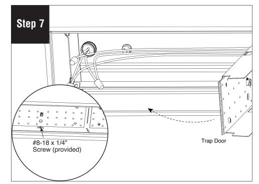
Make wire connections and secure trap door with #8-18 x 1/4" screw (provided).
