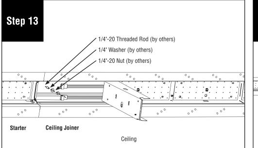
Install 1/4" washer (by others) and 1/4"-20 nut (by others) onto 1/4"-20 threaded rod (by others) or use alternate mounting option (use fastener and washer compatible to structural blocking to secure luminaire).
