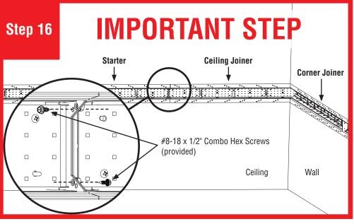
IMPORTANT STEP: Install 2 #8-18 x 1/2" combo hex screws (provided) into end bracket as shown. Screws can be installed from the left or right. CAUTION: Do not over-tighten.
