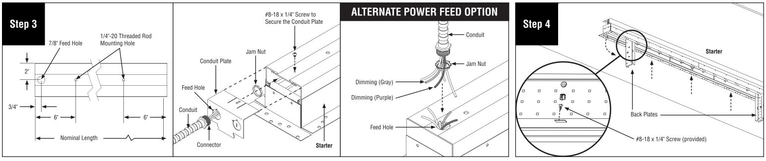
Refer to threaded rod and feed hole locations above before connecting luminaire wires. Remove jam nut from conduit then insert wires and connector through feed hole. NOTE: Purple and gray wires are for Low Voltage Control
