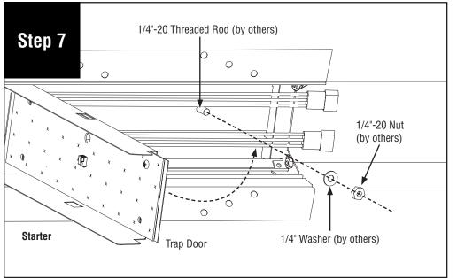
On opposite end of luminaire, install 1/4"-20 nut (by others) and 1/4" washer (by others) onto 1/4"-20 threaded rod (by others) or use alternate mounting option (use fastener and washer compatible to structural blocking to secure luminaire). Replace trap door and fasten with #8-18 x 1/4" screws (provided).
