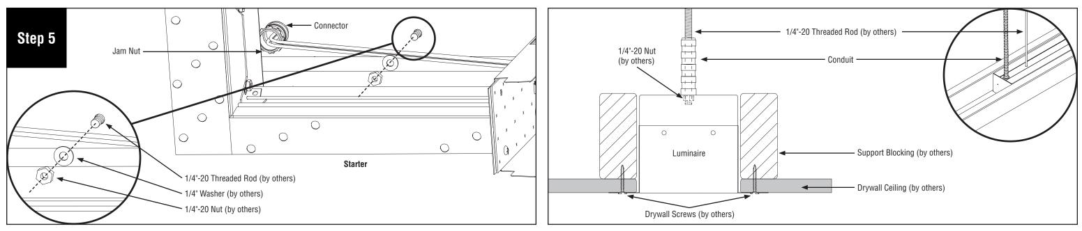
Install jam nut onto connector. Install 1/4"-20 nut (by others) and 1/4" washer (by others) onto 1/4"-20 threaded rod (by others).
