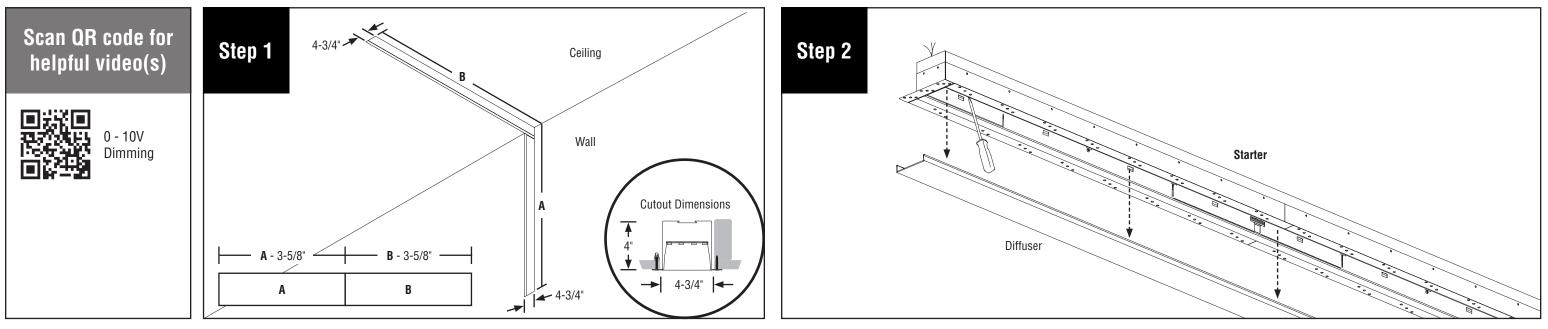
Subtract 3-5/8" from body/row length (A) and body/row length (B) to simplify installation. Luminaire needs to be installed next to support blocking. **NOTE:** Tolerances on dimensions are +/- 1/16". Please contact factory for dimensions of tailored luminaires with non-90° angles.
