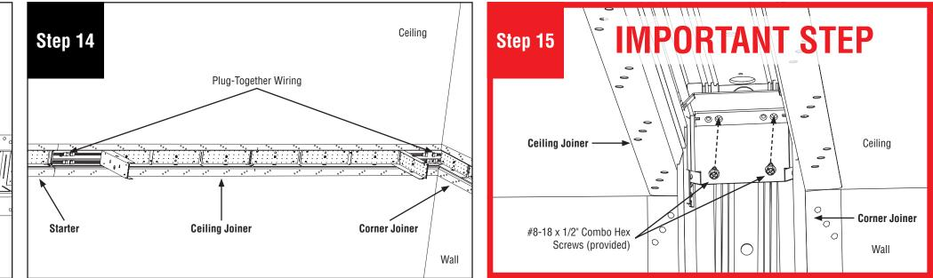
Connect plug-together wiring on both ends of the ceiling joiner luminaire.
