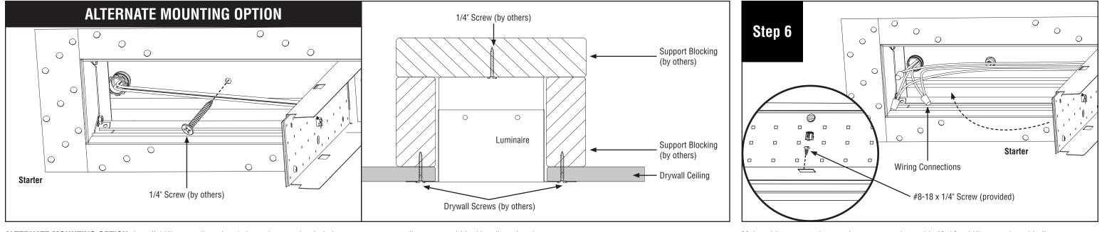
ALTERNATE MOUNTING OPTION: Install 1/4" screw (by others) through mounting hole into proper structurally supported blocking (by others).
