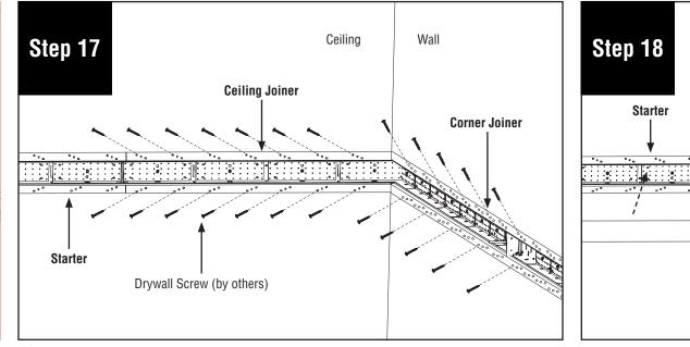
Fasten luminaires to the ceiling and wall with drywall screws (by others) through the flange into blocking.
