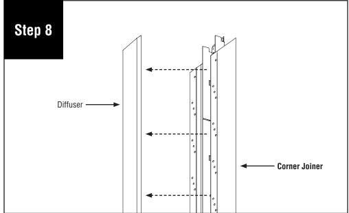
Remove diffuser from the corner joiner luminaire and set aside to prevent it from getting dirty or damaged.
