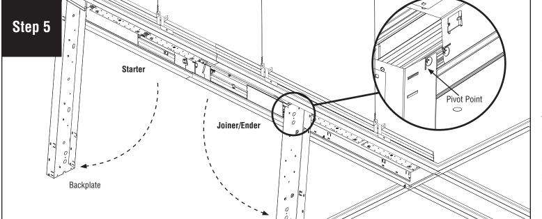
Slowly swing down backplates. **CAUTION: Do not twist the backplate when swinging down – it will come out of the support extrusion.** Note that the screws shown are the pivot points, and the backplate can be slid a few inches either way for ease of access to the driver space.
