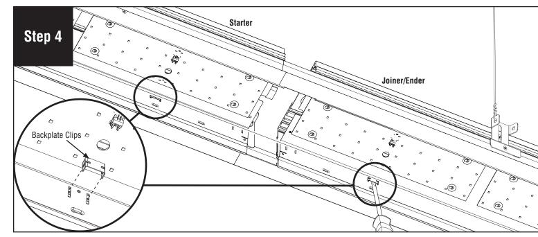
Remove backplate clips to release the backplates. We recommend using a flat head screwdriver to remove them. **CAUTION:** Do not lose these pieces.
