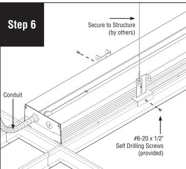
Secure luminaire to T-Bar with #6-20 x 1/2" self drilling sheet metal screw (provided).
