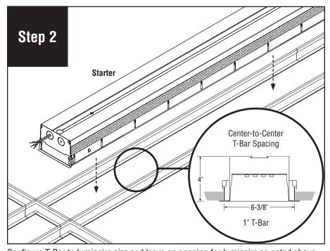
Configure T-Bar to luminaire size and leave an opening for luminaire as noted above. Make sure T-Bars are aligned at 90 degrees. Place luminaire on T-Bar.
