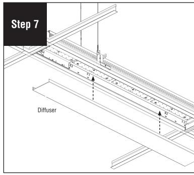
Reinstall diffuser and turn power on. **NOTE:** If part of a longer run, reinstall diffuser back into the original luminaire section as lengths vary.
