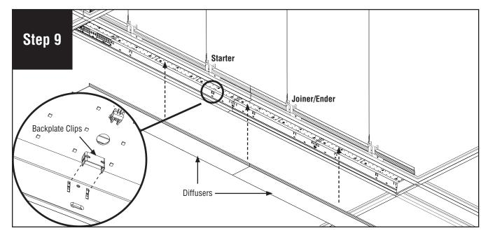
Replace backplates by holding them in their original position and pushing the clips back in. Make sure wire connections are not pinched. (If a 1 ft. backplate assembly is near joint, reconnect feed harness to LED board.) Replace diffuser and turn power onto luminaire. NOTE: If part of a longer run, diffuser will be reinstalled back into original luminaire section as lengths vary.
