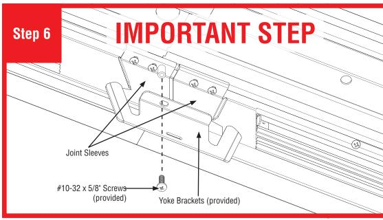
IMPORTANT STEP: Secure joint with two yoke brackets (provided) using two #10-32 x 5/8" screws (provided). When installed correctly these brackets will pull luminaires together to make a tight joint. CAUTION: Do not over-tighten.
