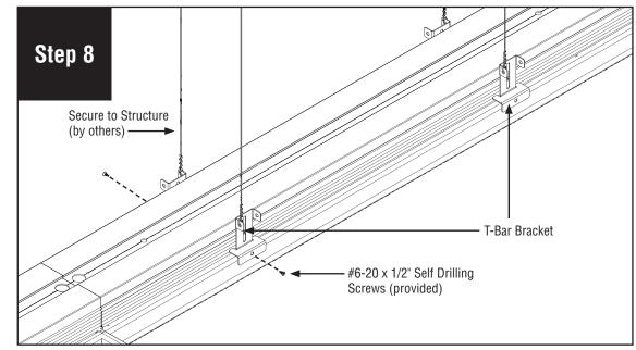
Secure luminaire to T-Bar with #6-20 x 1/2" self drilling sheet metal screw (provided).
