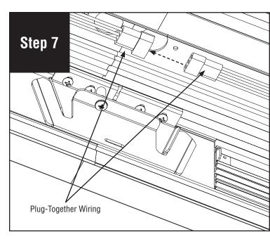
Connect-plug together wiring connections.
