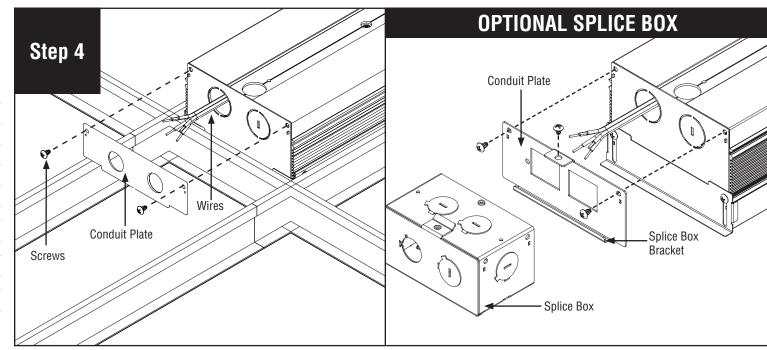
Remove conduit plate from luminaire. **NOTE:** Purple and gray wires are for Low Voltage Control.
