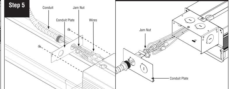
Run power cables through conduit plate and jam nut. Make electrical connections. Secure conduit onto conduit plate with jam nut, and reinstall conduit plate carefully not to damage any wiring.
