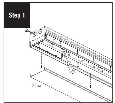
Remove diffuser and set aside to prevent it from getting dirty or damaged. NOTE: If part of a longer run, diffuser will be reinstalled back into original luminaire section as lengths vary.
