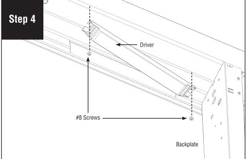
Remove #8 screws that attach the driver to the body screw channels. Disconnect all wiring from the driver.
