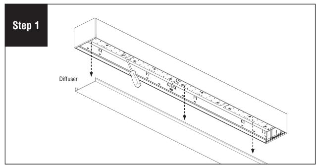
Remove diffuser and set aside to prevent it from getting dirty or damaged. **NOTE:** If part of a longer run, diffuser will be reinstalled back into original luminaire section as lengths vary.
