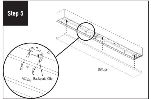
Replace new driver and reconnect all wiring. Replace backplate by returning it to its original position and reinstalling the backplate clips. Replace diffuser and turn on power to luminaire.
