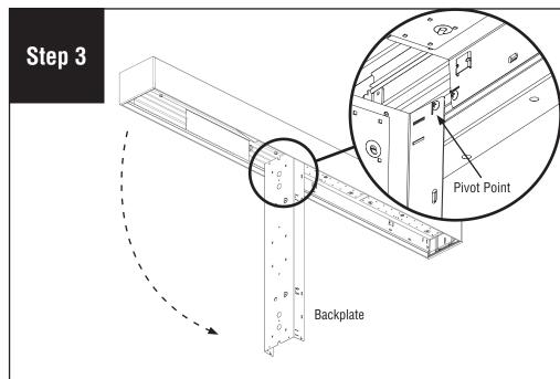
Slowly swing down backplate. CAUTION: Do not twist the backplate when swinging down - it will come out of the support extrusion. Note that the screws shown are the pivot point, and the backplate can be slid a few inches either way for ease of access to the driver space.
