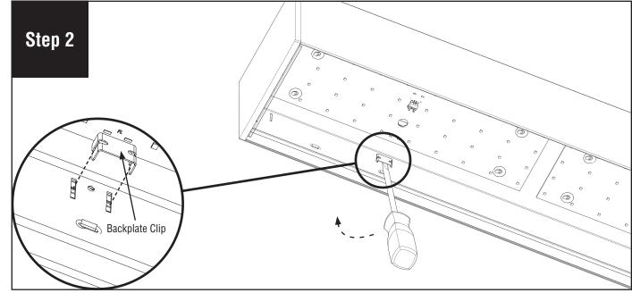
Remove backplate clips to release the backplate. We recommend using a flat head screwdriver to get them loose. CAUTION: Do not lose these pieces.
