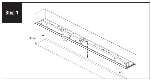
Remove diffuser and set aside to prevent it from getting dirty or damaged. **NOTE:** If part of a longer run, diffuser will be Disconnect the feed harnesses from LED boards. reinstalled back into original luminaire section as lengths vary.
