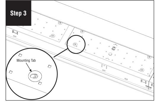
Shift LED board away from the Mounting Tab. Bend tabs open if needed.
