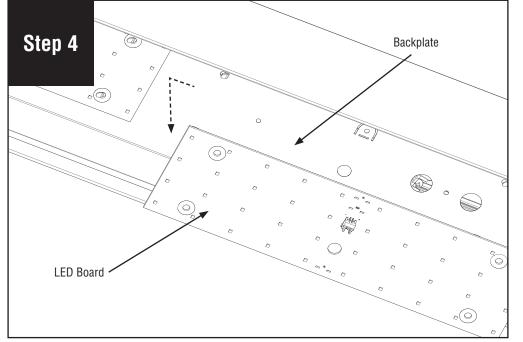
Lift LED board away from the back plate. Replace new LED board, bend tabs down to secure. Reconnect feed harnesses. Reinstall diffuser and turn power on to luminaire.
