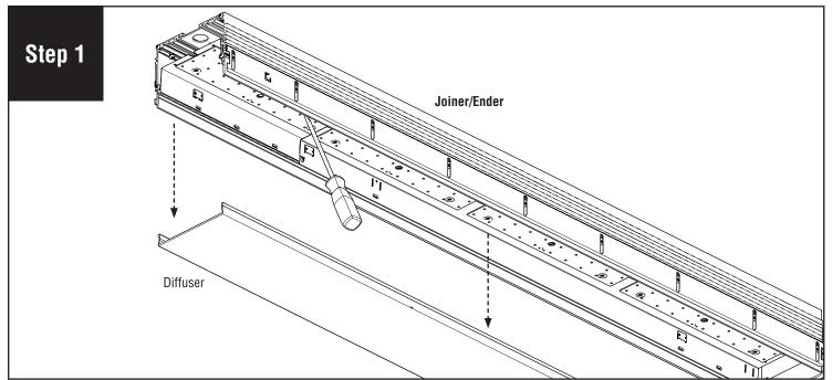
Remove diffuser and set aside to prevent it from getting dirty or damaged. **NOTE:** If part of a longer run, diffuser will be reinstalled back into original luminaire section as lengths vary.
