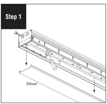
aged. **NOTE:** If part of a longer run, diffuser will be reinstalled back into original luminaire section as lengths vary.
