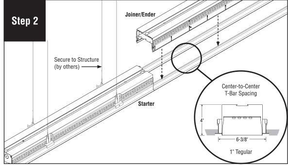
Install joiner/ender onto ceiling next to starter. Align the starter and joiner/ender luminaires and slide them together.
