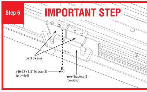
**IMPORTANT STEP:** Secure joint with two yoke brackets (provided) using two #10-32 x 5/8" screws (provided). When installed correctly these brackets will pull luminaires together to make a tight joint.
