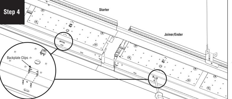
Remove backplate clips to release the backplates. We recommend using a flat head screwdriver to remove them. **CAUTION:** Do not lose these pieces.
