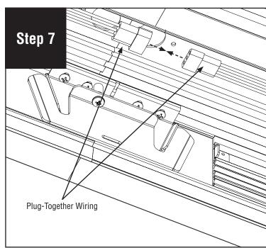
Connect plug-together wiring connections.
