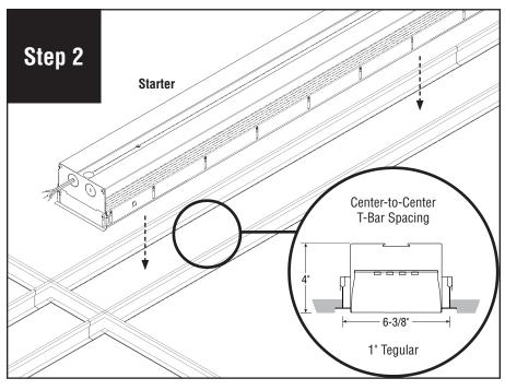
Remove diffuser and set aside to prevent it from getting dirty or dam- Configure T-Bar to luminaire size and leave an opening for luminaire as noted above. Make sure T-Bars are aligned at 90 degrees. Place luminaire on T-Bar.
