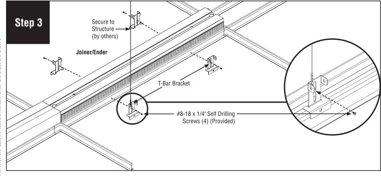
Install T-Bar bracket onto luminaire. Secure with #8-18 x 1/4" screws (provided). Secure luminaire to structure using tie-wire (by others), as per code.
