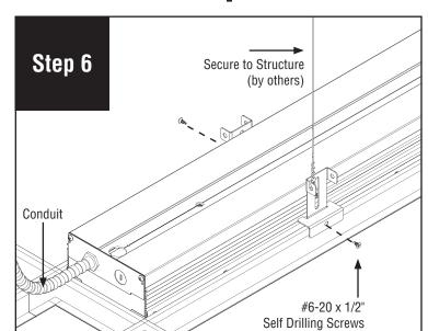
Secure luminaire to T-Bar with #6-20 x 1/2" self drilling sheet metal screw (provided).
