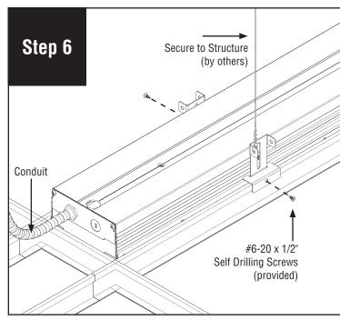
Secure luminaire to T-Bar with #6-20  $\times$  1/2" self drilling sheet metal screw (provided).
