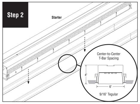
Configure T-Bar to luminaire size and leave an opening for luminaire as noted above. Make sure T-Bars are aligned at 90 degrees. Place luminaire on T-Bar.
