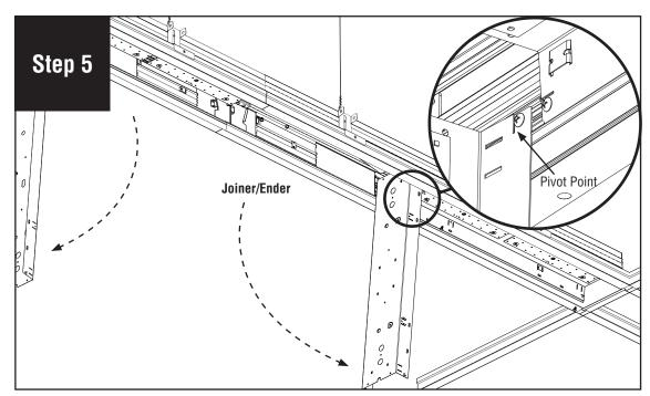
Slowly swing down backplate. **CAUTION:** Do not twist the backplate when swinging down – it will come out of the support extrusion. Note that the screws shown are the pivot points, and the backplate can be slid a few inches either way for ease of access to the driver space.
