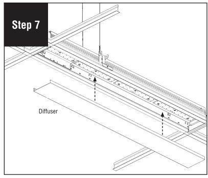
Reinstall diffuser and turn power on. **NOTE:** If part of a longer run, diffuser will be reinstalled back into original luminaire section as lengths vary.
