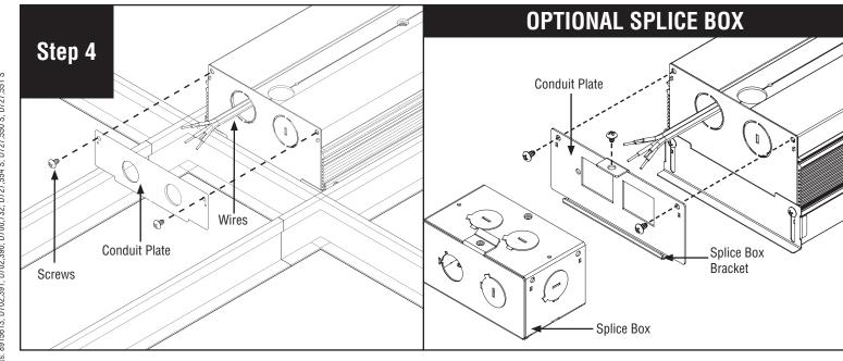
Remove conduit plate from luminaire. **NOTE:** Purple and gray wires are for Low Voltage Control.
