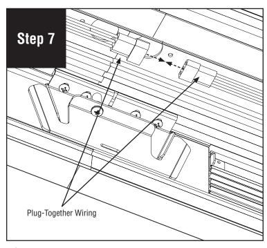
Connect plug-together wiring connections.
