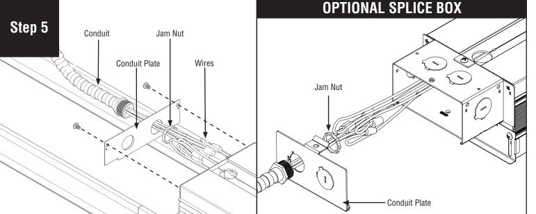
Run power cables through conduit plate and jam nut. Make electrical connections. Secure conduit onto conduit plate with jam nut, and reinstall conduit plate carefully not to damage any wiring.
