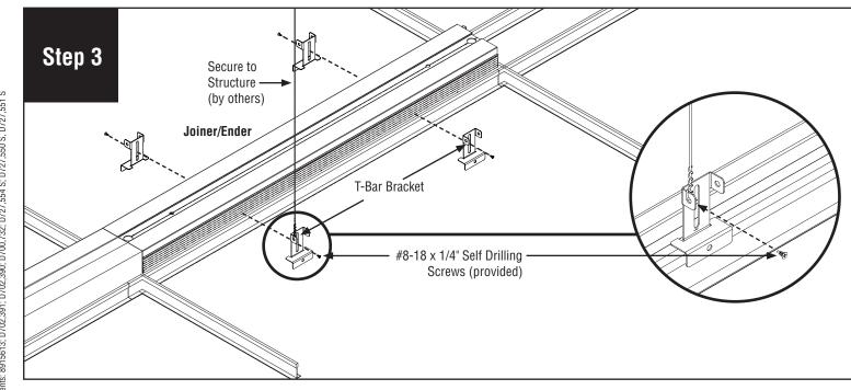
Install T-Bar bracket onto luminaire. Secure with #8-18 x 1/4" screws (provided). Secure luminaire to structure using tie-wire (by others), as per code.
