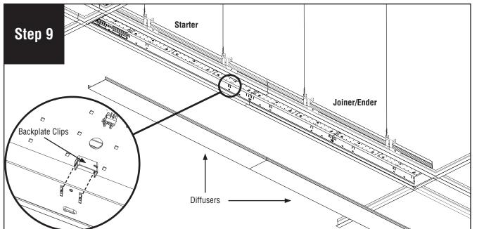
Replace backplates by holding them in their original position and pushing the clips back in. Make sure wire connections are not pinched. (If a 1ft. backplate assembly is near joint, reconnect feed harness to LED board.) Replace diffuser and turn power on to luminaire. **NOTE:** If part of a longer run, diffuser will be reinstalled back into original luminaire section as lengths vary.
