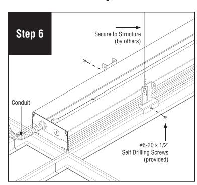
Secure luminaire to T-Bar with #6-20 x 1/2" self drilling sheet metal screws (provided)
