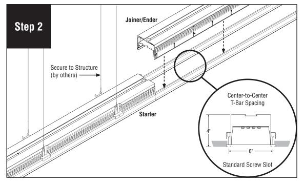
Remove diffuser from Joiner/ Ender and set aside to prevent it from getting dirty or damaged. NOTE: If part of a longer run, diffuser will be reinstalled back into original luminaire section as lengths vary.
