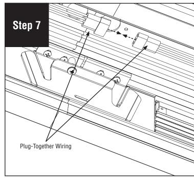
Connect plug-together wiring connections.
