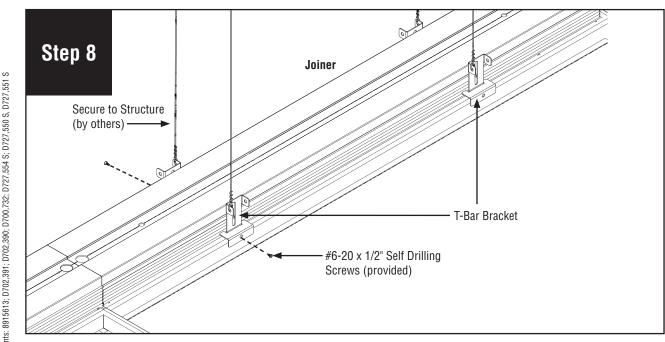
Secure luminaire to T-Bar with #6-20 x 1/2" self drilling sheet metal screws (provided)
