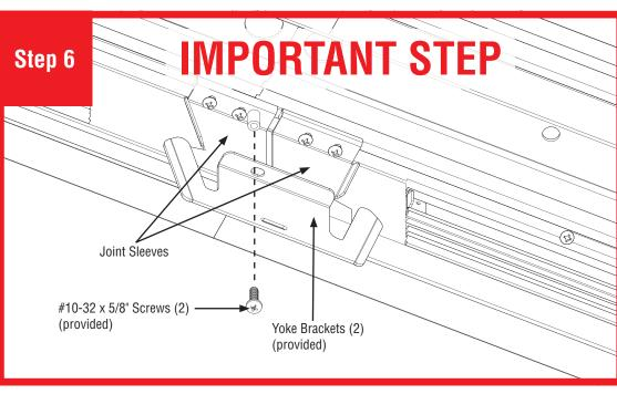
IMPORTANT STEP: Secure joint with two yoke brackets (provided) using two #10-32 x 5/8" screws (provided). When installed correctly these brackets will pull luminaires together to make a tight joint. CAUTION: Do not over-tighten
