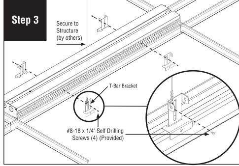
Install T-Bar brackets onto luminaire. Secure with #8-18 x 1/4" screws (provided). Secure luminaire to structure using tie-wire (by others), as per code.
