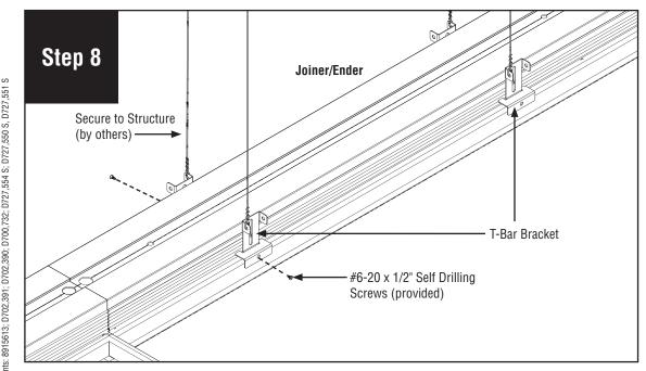
Secure luminaire to T-Bar with #6-20 x 1/2" self drilling sheet metal screws (provided).
