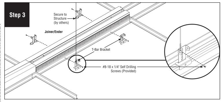
Install T-Bar brackets onto joiner/ender luminaire. Secure with #8-18 x 1/4" screws (provided). Secure luminaire to structure using tie-wire (by others), as per code.
