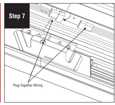
Connect plug-together wiring connections.
