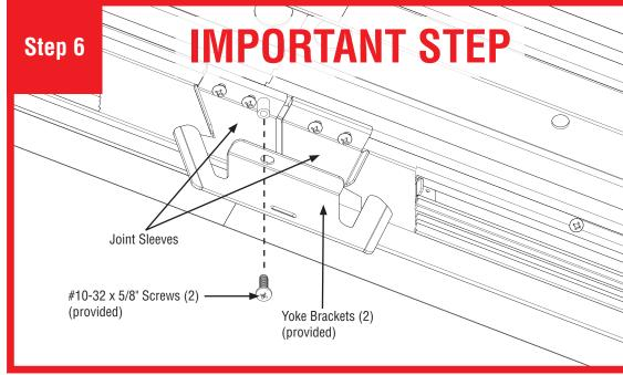
**IMPORTANT STEP:** Secure joint with two yoke brackets (provided) using two #10-32 x 5/8" screws (provided). When installed correctly these brackets will pull luminaires together to make a tight joint. **CAUTION: Do not over-tighten.**
